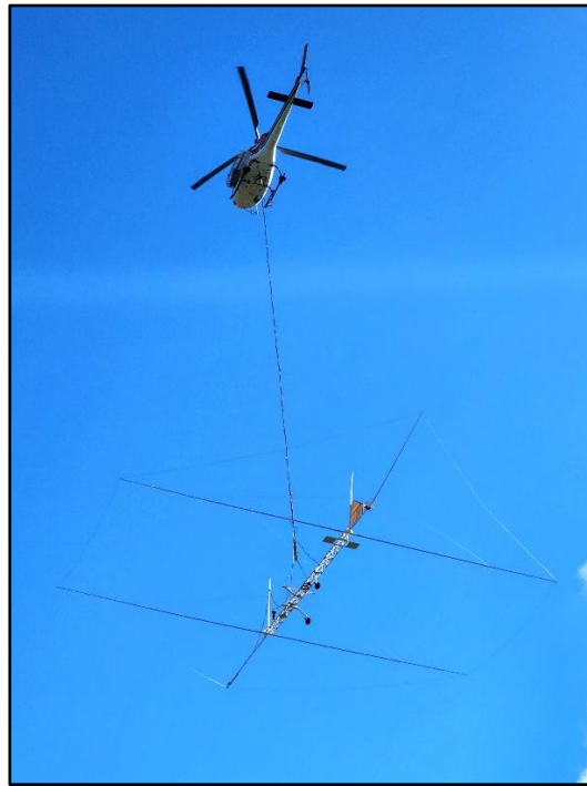
Figure 10: 1TEM structure with a single wrap of the transmitter loop.
