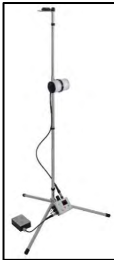
Figure 9: Geodevice SmartMag Overhauser magnetometer.
